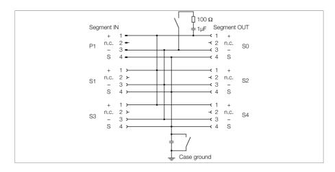
The 4-channel junction box JBBS-48-E413/3G is designed for PROFIBUS-PA systems.
