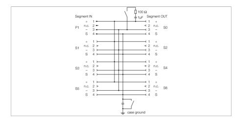
The 6-channel junction box JBBS-48-E613/3G is designed for PROFIBUS-PA systems.
