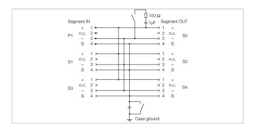
The 4-channel junction box JBBS-48-M413/3G is designed for PROFIBUS-PA systems.
