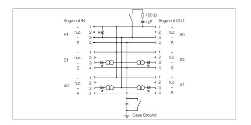
The 4-channel junction box JBBS-48SC-E413/3G is designed for PROFIBUS-PA systems.
