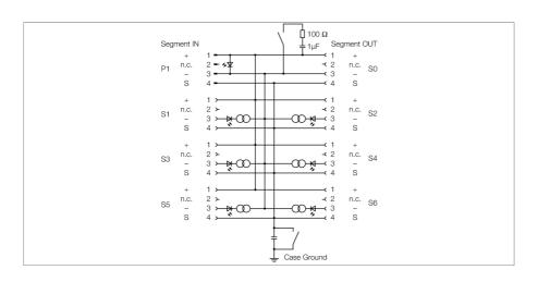
The 6-channel junction box JBBS-48SC-E613/3G is designed for PROFIBUS-PA systems.
