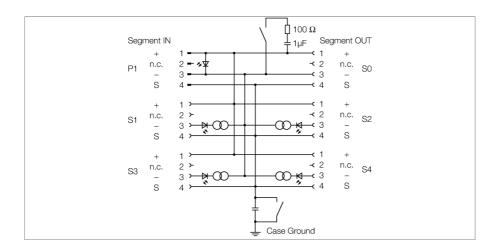
The 4-channel junction box JBBS-48SC-M413/3G is designed for PROFIBUS-PA systems.
