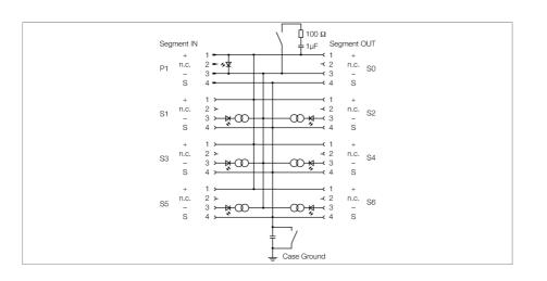
The 6-channel junction box JBBS-48SC-M613/3G is designed for PROFIBUS-PA systems.
