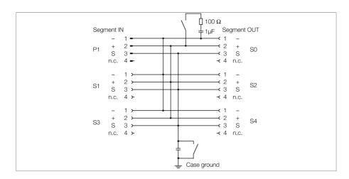
The 4-channel junction box JBBS-49-M413/3G is designed for FOUNDATION™ fieldbus systems.
