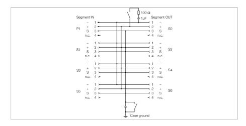
The 6-channel junction box JBBS-49-M613/3G is designed for FOUNDATION™ fieldbus systems.
