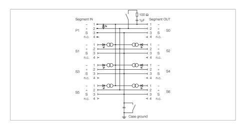
The 6-channel junction box JBBS-49SC-E613/3G is designed for FOUNDATION™ fieldbus systems.
