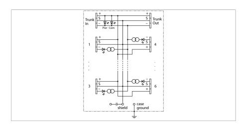
The junction box is designed for fieldbus systems acc. to IEC 61158-2, i.e. it is suited for both FOUNDATION™ fieldbus and PROFIBUS-PA. When connected to a suitable power supply unit, it can also be used in Ex applications.
