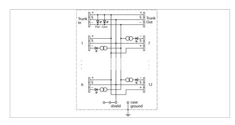
The junction box is designed for fieldbus systems acc. to IEC 61158-2, i.e. it is suited for both FOUNDATION™ fieldbus and PROFIBUS-PA. When connected to a suitable power supply unit, it can also be used in Ex applications.
